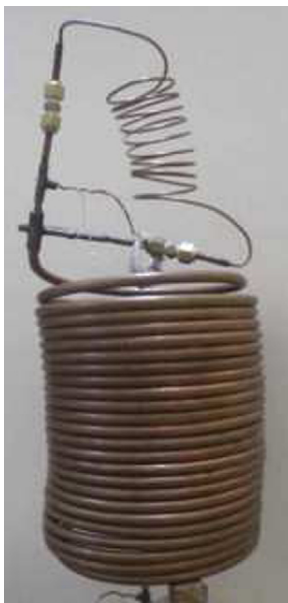
Fig. 3. Photograph of the heat exchanger [18].
